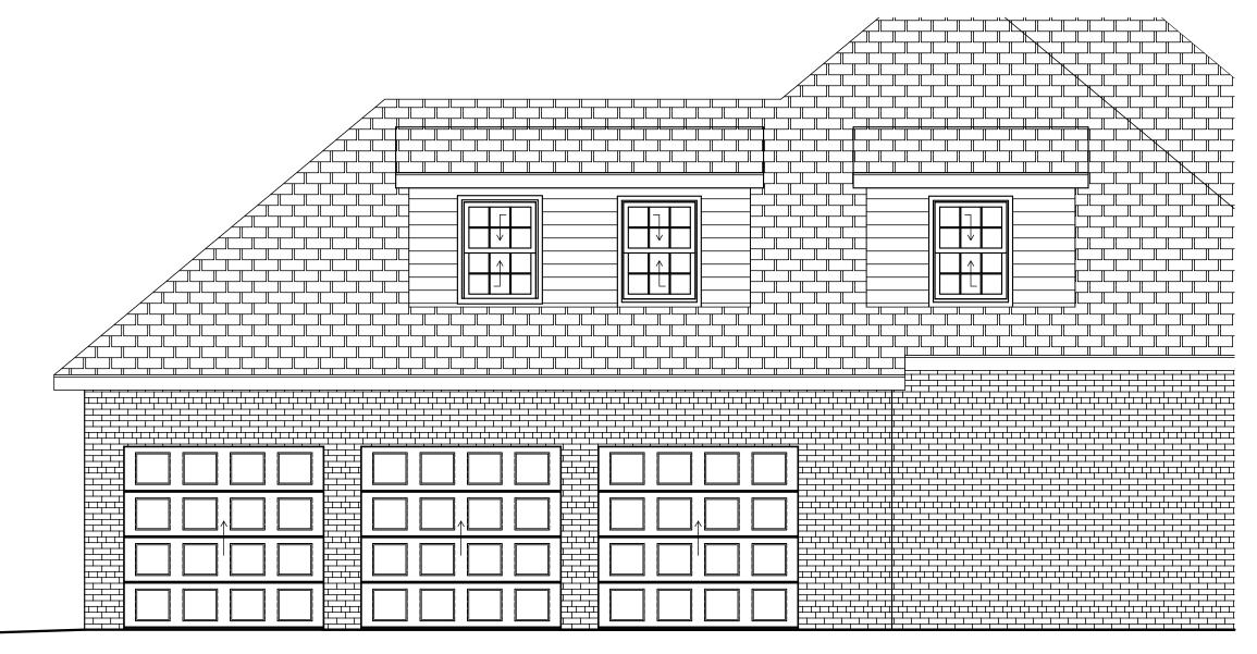
**NOTE:** Elevation is diagrammatic and meant to illustrate location of the new second floor dormers. Exact details and finishes to be determined by client and contractor.
