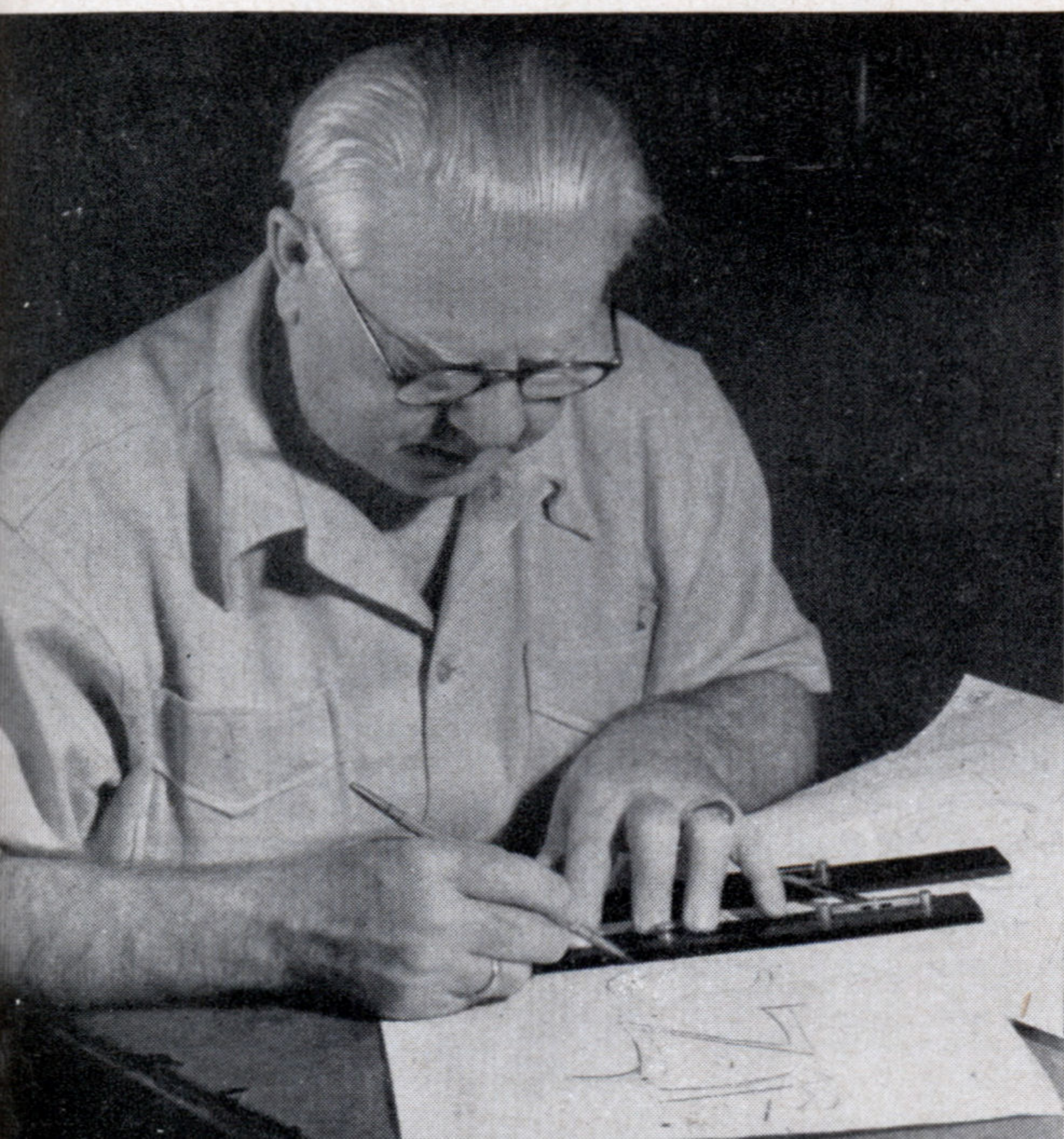
Birth of a new type face: Goudy first lays out five guide lines to fix the upper and lower limits of the various kinds of letters. Then, with sharp-pointed pencils, he draws the letters. Drawings are 7½ inches tall. Pinholes mark the important points in each design as a guide for the next step—transferring it onto draftsman's cardboard
